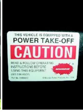
Follow the PTO manufacturer's operating instructions to operate the PTO properly for your vehicle Note that driving with the PTO engaged may damage both the hydraulic pump and the PTO.
