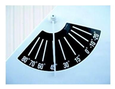
The boom angle indicator shows 45 degrees. In the "angle" column locate 45 degrees and follow it across to the "second and third sections extended" boom configuration to determine the load radius and sheave height. In our example, the load radius is 23.4 feet and sheave height is 32.7 feet.
