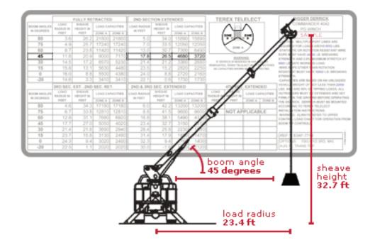
A diagram on the load chart illustrates the zones around the truck, from which load capacities are determined. Since the load is positioned in Zone B, we will look under the "Zone B" column to find that our boom capacity is 2,510 pounds.
